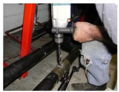
7 Drill out the 3 dimples in each tube (using a 14 mm drill) in the center of the axle This will allow rotation of internal clamp.
