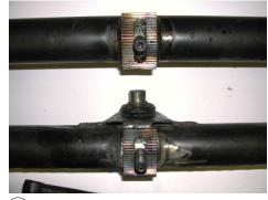
(1) This photo shows the two bolts at half way position prior to refitting in the bus. Final adjustment can then be made.
