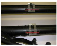
The lowest part of your adjustors slot, should be where the original lock bolt was located. Adjustment will be upwards to lower the bus.
