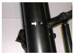
6 There are 3 dimples in each tube. These lock The internal spring clamp.
