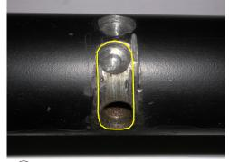
(10) You now must remove the material within the area shown above. Drill the top hole and then make two vertical cuts with a hacksaw.
