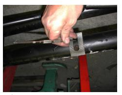
Scribe around the inside of the slot with the original internal locking bolt hole at the bottom of the slot.
