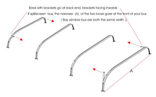
Einger tighten the cap head screws into alloy uprights. Use M4 machine screws and nylocs to secure wood .
