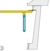
With the window secured with screws, attach the slides to the bracket on the frame.
