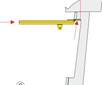
With the window centred on the marks A & B, carefully open the Safari ready to scribe through the holes in the hinge. Before you scribe the hole positions, be sure to push the window into the aperture so that the hinge "bottoms out" at the back of the recess D. Keeping the frame centred on A& B, scribe the hole locations. Drill the holes using a 2mm drill bit. When you have drilled them all, open up preferably to 2.5mm or 3mm. The 2.5drill will give more grip to the screws.
