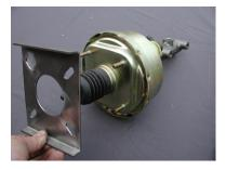
This photo shows the relationship between the Servo assembly and the steel mount which must be welded to your front beam.
