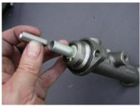
Close up of bullet being fitted with pointed end inserted first.
