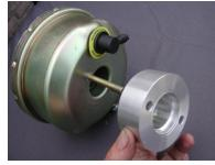
Slip Alloy spacer onto two studs, making sure that recess faces away from servo.
