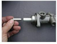
It is **VITAL** that you insert the bullet push rod pointed radius first, inside your T2 Servo Master cylinders (611 021 211) hollow push rod tube.
