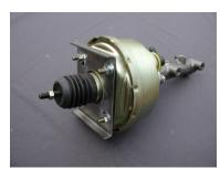
Servo assembly is secured to folded bracket by M8 nylocs and washers.
