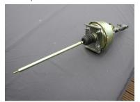
This photo shows the push rod fitted to the assembly. It is a good idea to hold the assembly up under your bus to test for clearance before welding on the bracket.
