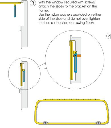
With the window secured and the slide attached, you can now fit the body bracket.
