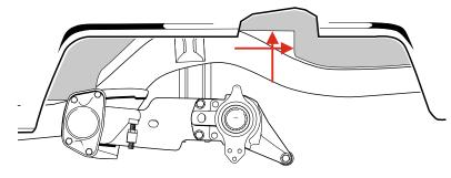
The shock mount is designed to fit in the floor corner underneath the fuel tank floor area. See above diagram. It should be positioned as high and rearward into the corner shown and will self locate.
