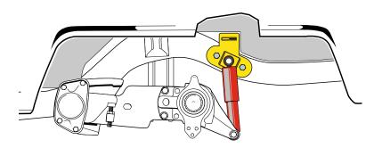
When you have drilled through your chassis, secure with the supplied fasteners. The completed installation should look like this. Be sure to use the correct length shock which can only be calculated with the vehicle on the ground under full weight. The bolt to bolt measurement will be required to select the right length shock. See our attached chart, Pick up trucks require the mount to be fitted at a slight angle.
